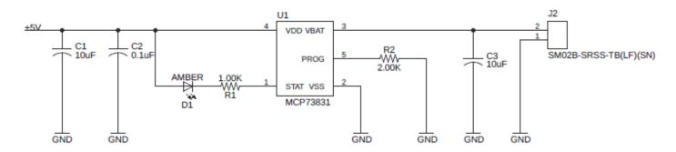
Figure 3: Sample Battery Charger Schematic
